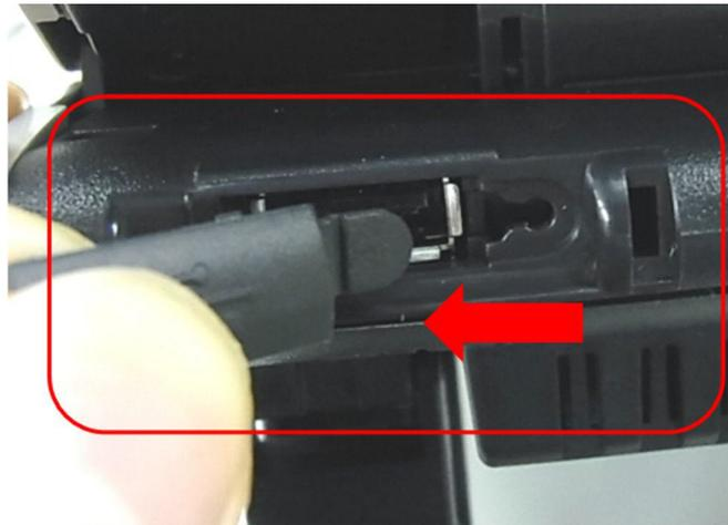
**Note:** Do not pull the cover upward. If the USB Port Cover is pulled upward, the cover may rip apart from the connector.
